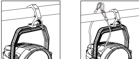
灯钩吊挂图 Hanging with Clamp 安全链吊挂图 Hanging with Safety Cable
